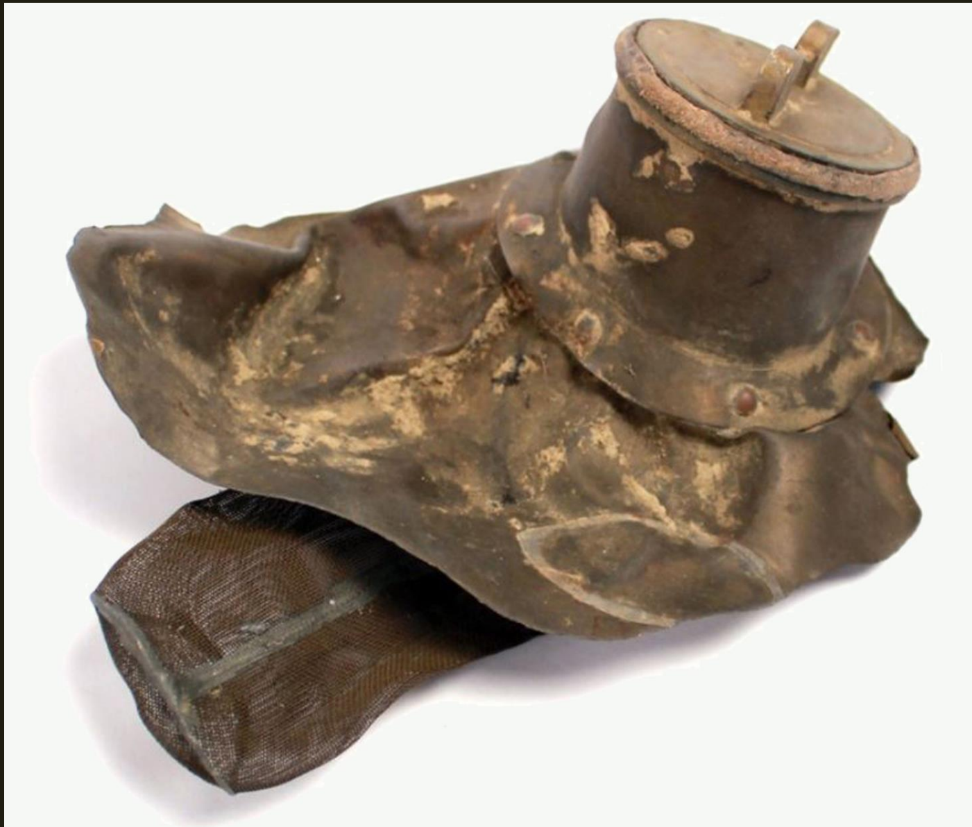
The brass fuel cap and its fine mesh screen which tore away from the tank in the crash. Credit: Xavier Aiolfi
