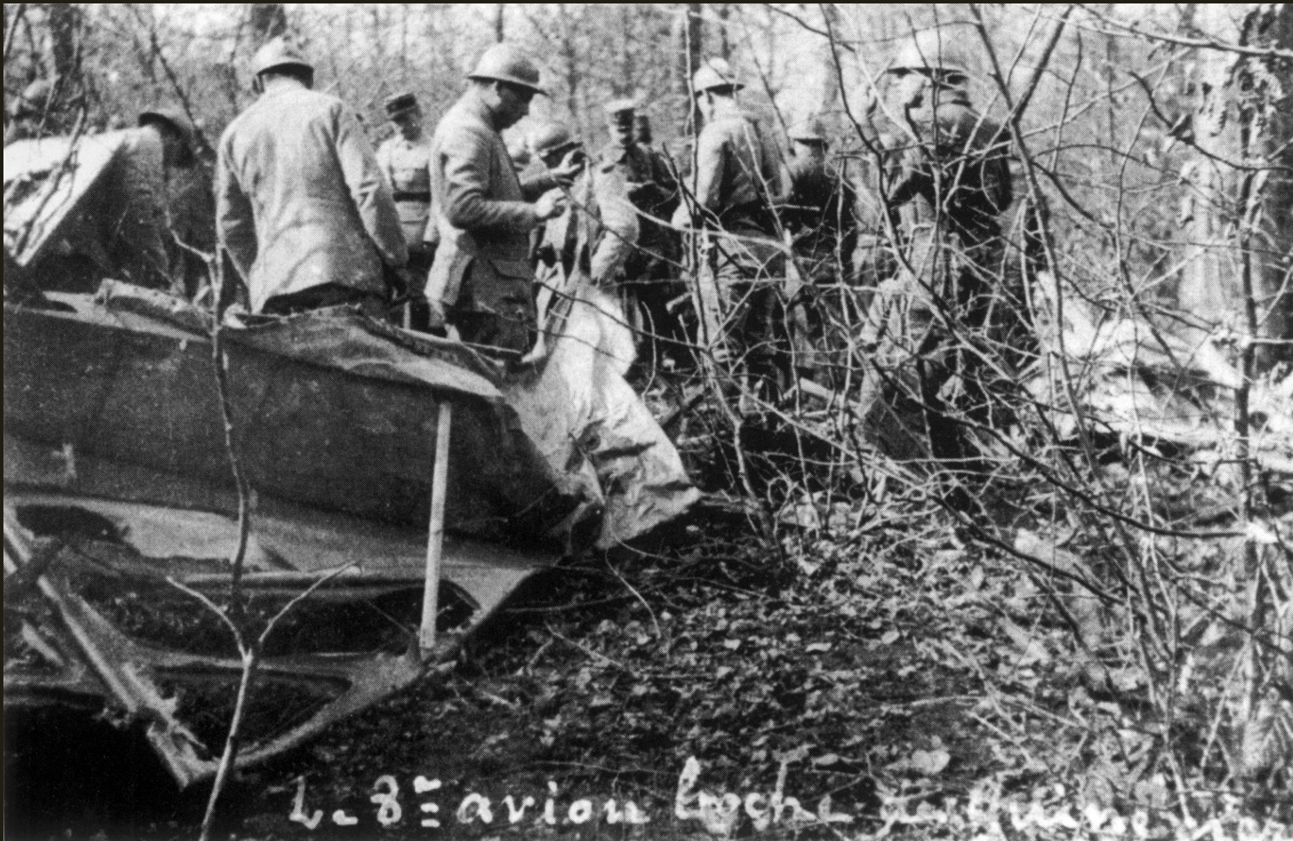
The fuselage broken into 2 pieces- the rear third of the aircraft lies upside down. Courtesy of Greg VanWyngarden
