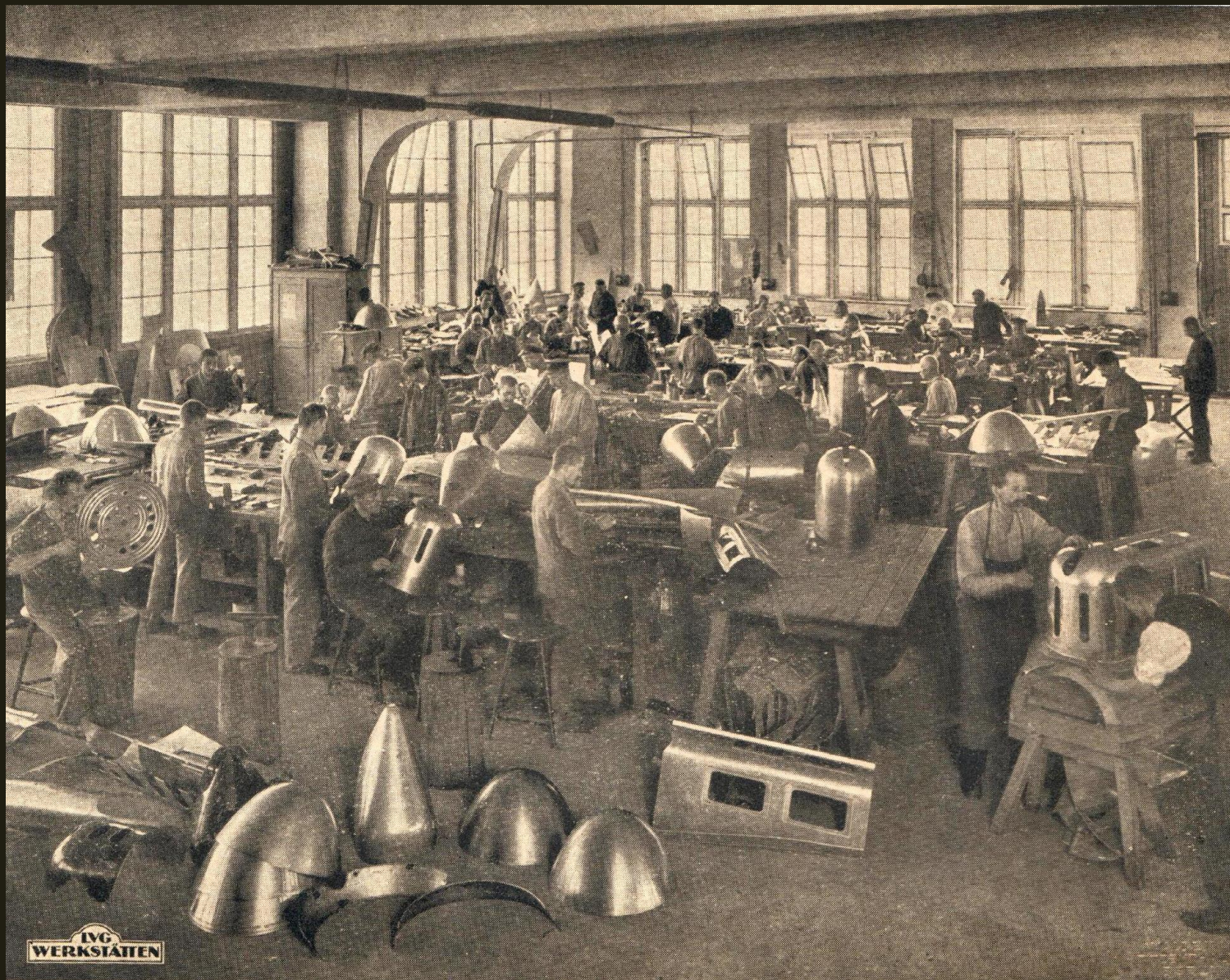
“Montage-Klempner” or Assembly-Plumber, the part of LVG’s factory where tanks were fabricated. Photo courtesy of Peter Cohausz, source: Das Flugzeug Vergangenheit Gegenwart Zukunft , LVG Company, 1919.
