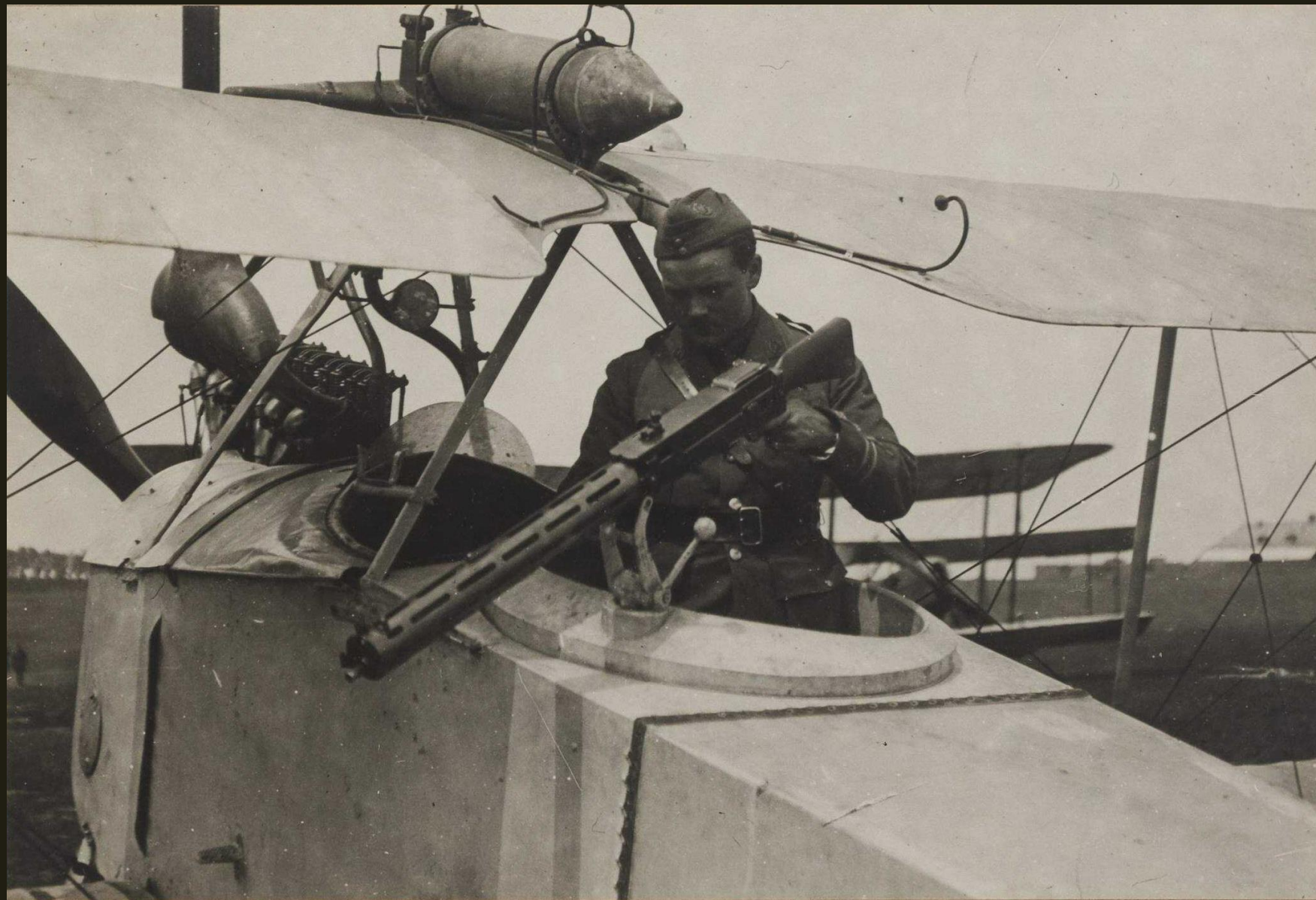
An R.F.C. officer inspects the observer's gun on an LVG CII captured by the French and extensively photographed and tested at Villacoublay, the French aviation test center, in June, 1916. The gravity-fed reserve tank is seen on the top wing with its aerodynamic design. Courtesy of Bibliothèque de documentation internationale contemporaine
