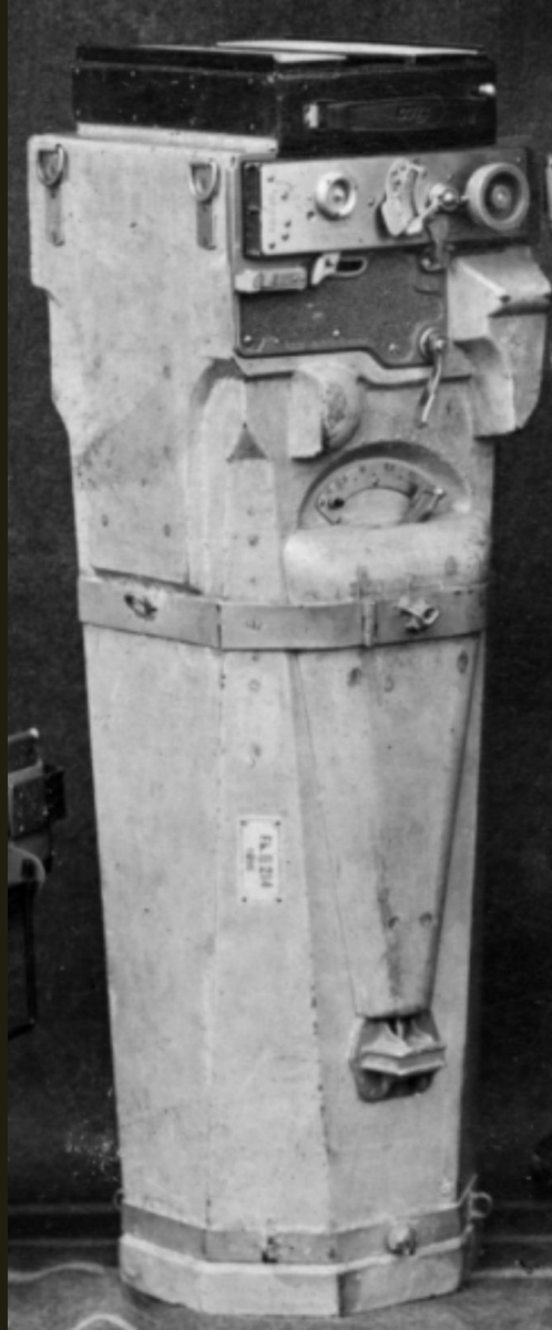
Photo of a Fliegerkamera II , 50cm, as identified by Terry Finnegan
